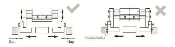
7.2) The end of stroke under the move state of air gripper
