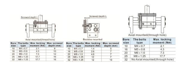
6. The installation method of the gripping jaw fittings When install the gripping jaw fittings, you have to pay particular attention that you can only hold the gripping jaw by using spanner, and then lock the screws with allen wrench. Never clamp the body directly and then lock the screws, otherwise the parts will be easily damaged.
