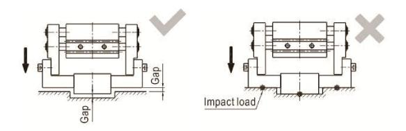
8. When the work-pieces are inserted, the center line should be coaxial, no offset, in case there are external force generated on gripping jaw. When testing, it is specially required that the manual operation should be reduced, the pressure should be used to run it at a low speed, and guarantee the safety and no impact.
