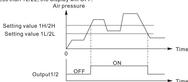
3. Window comparator mode: Set the pressure value H/L. When the pressure is greater than the H value or less than the L value, the output is OFF; when the air pressure is greater than the L value and less than the H value, the output is ON.
